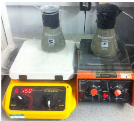
Figure 87: From Batch test #5 (x4 months), Synthetic groundwater batch test set up for 150°C, right; distilled water+ steel coupon, left; Synthetic groundwater+ steel coupon
