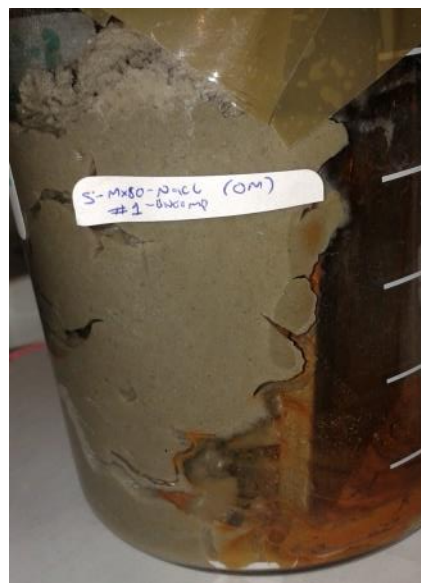
Figure 85: From Batch test #3 (x1 month Steel/Mx-80 & increasing saline solution), C-Steel plate in contact with uncompact Bentonite
