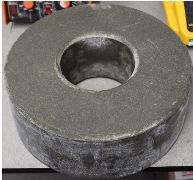
Figure 90: Pre- compacted Bentonite block supplied by ClayTechAB®, used in the interface exposure experiments
