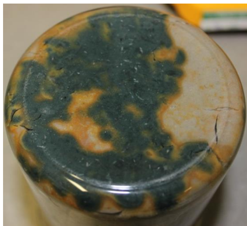
Figure 88: From Batch #6 (Steel/Mx-80 & distilled water), C-Steel plate in contact with uncompact Bentonite at 20°C for 1 year
