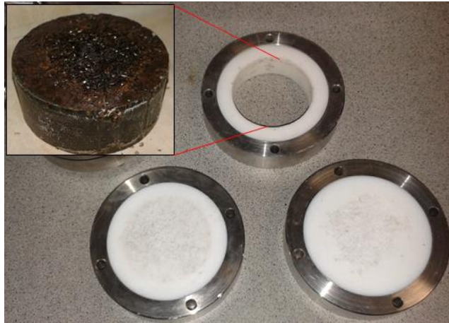
Figure 86: From Batch test #4 (x1 month Steel/Mx-80 & distilled water), compacted and heated to 100°C within a constant volume cell
