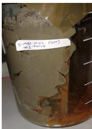
Figure 155: From batch #4 (Steel/Mx-80 & increasing saline solution), C-Steel plate in contact with uncompact Bentonite (DI water sample)
