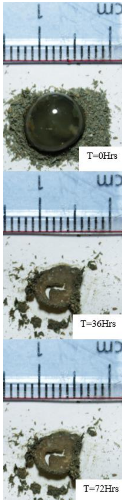
Figure 208: Time-lapse pictures of the hydrated oxidation tests
