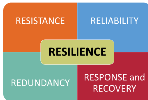
Figure 2-4. The four components to be considered when evaluating infrastructure resilience, according to the Cabinet Office (2011).
