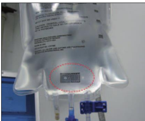
Figure 2.57. Graphene wireless sensor for S. Aureus bacteria detection attached on an intravenous bag [365].
