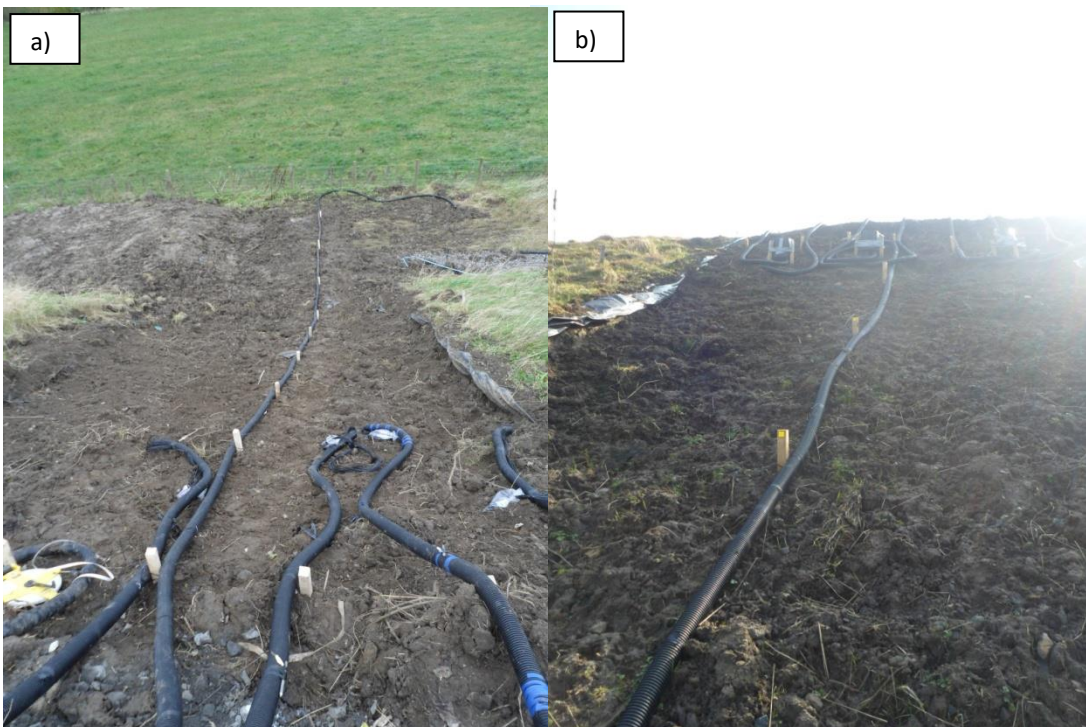
Figure 4.44 North flank of ERT test plot, showing long central line. View from (a) crest, and (b) North toe
