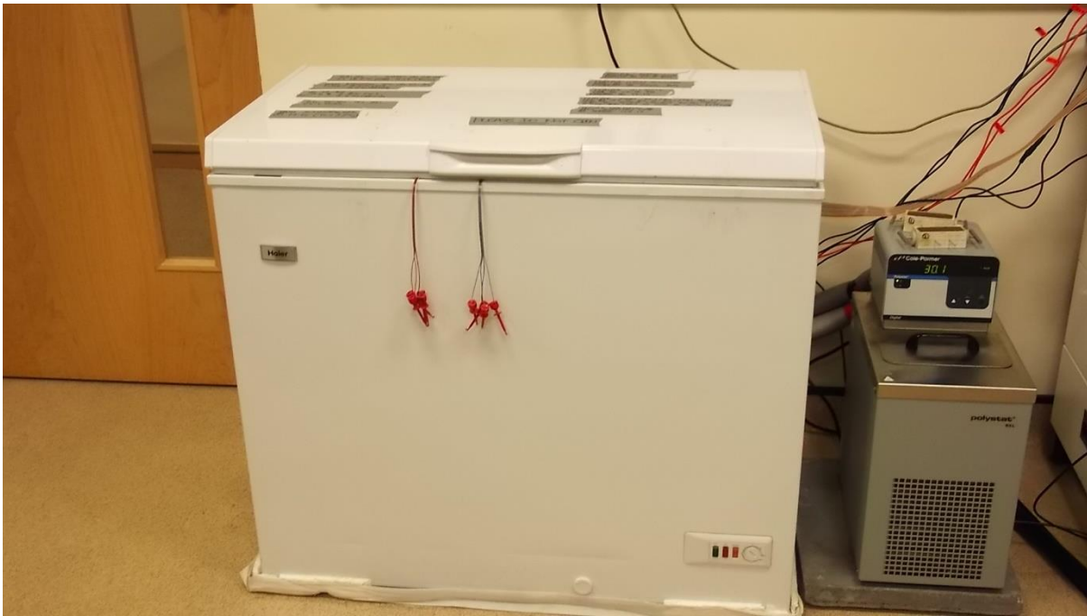
Figure 4.24 Insulated heating chamber and Polystat heat generator
