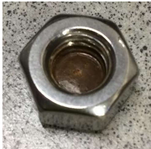
Figure 4.29 Steel nut filled to a depth of 5 mm
