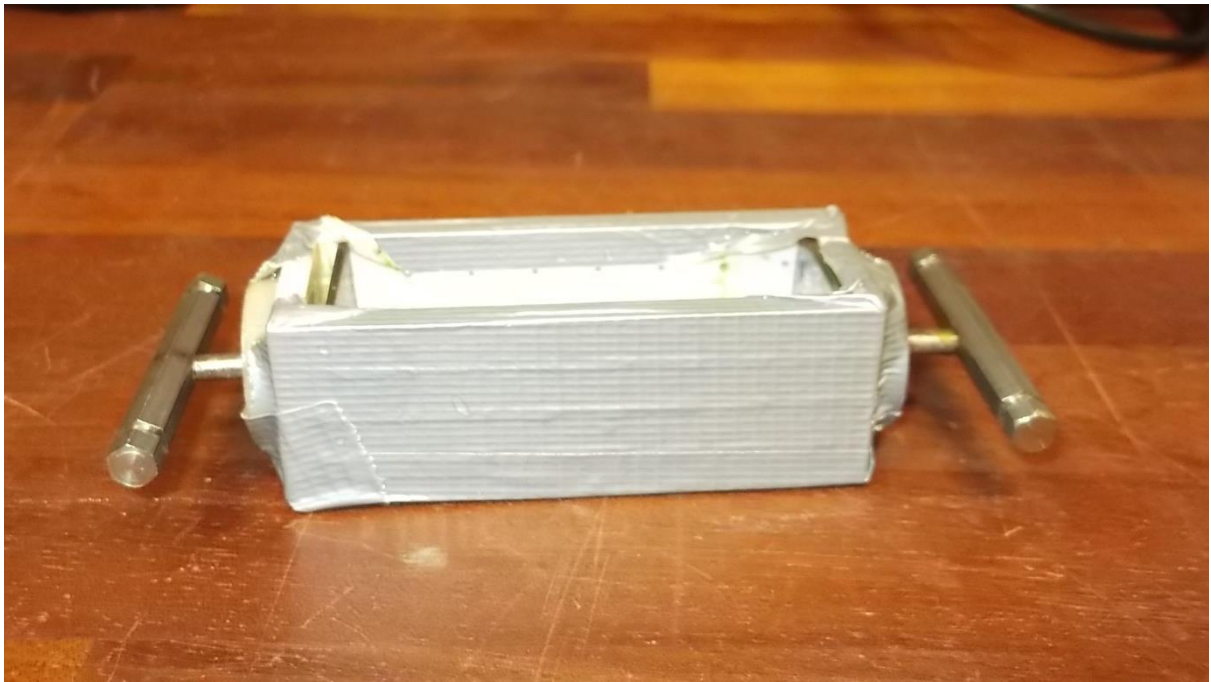
Figure 4.21 Waterproofing of resistivity test chamber for derivation of geometric factor
