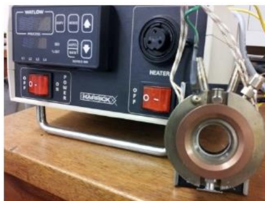
Figure 2. High-temperature cell and the temperature controller used in this work.
