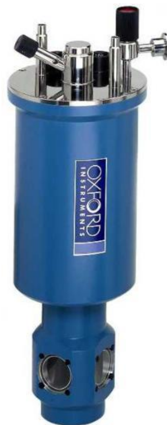
Figure 1. Photograph of the cryostat used for low-temperature studies.
