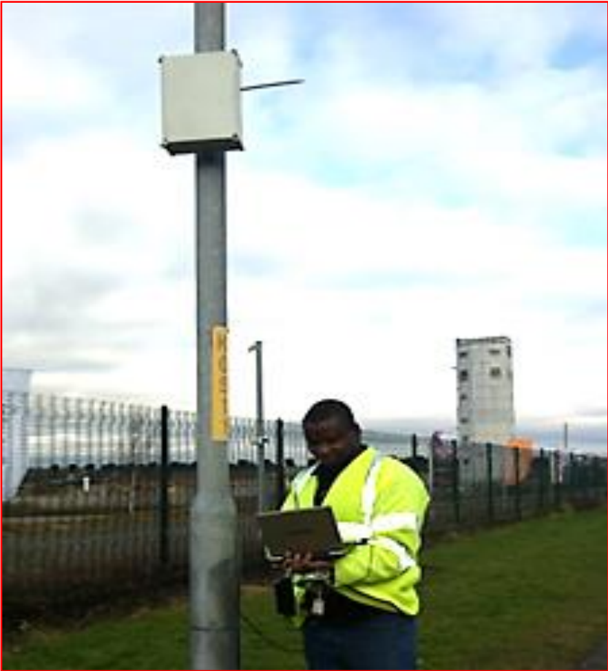
Appendix 1: A typical Bluetooth sensor mounted on a lamp post
