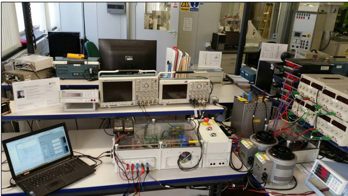
Figure 6.1. Test rig for experimental grid-connected PV inverter system.
