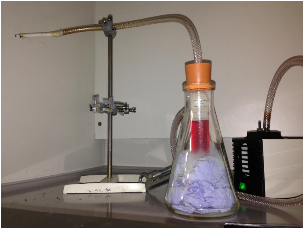
Figure 2.1 Set up of equipment used to generate cigarette smoke extract.
