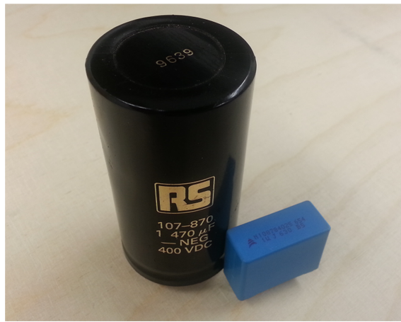
Figure 4.37: Photo showing the size difference between a 1\mu\text{F} 630V film capacitor and a 470\mu\text{F} 400V electrolytic capacitor
