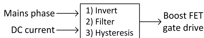
Figure 6.2: Control functions for the filter-based APFC system
