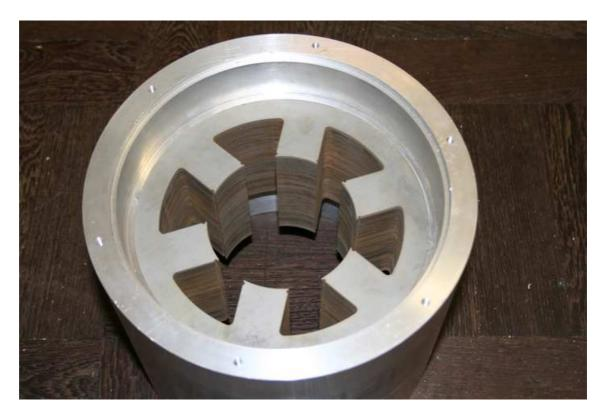
Figure 7.2: Stack of Stator Lamination in the Case
