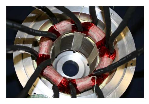
Figure 7.7: Tying Cords, Heat Shrinks and Thermal Coupling
