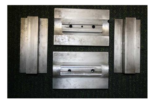
Figure 7.4: Coil Forming Bobbin
