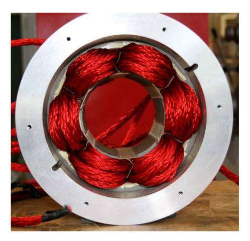
Figure 7.6: Coils, Nomex and Tufnol Insulations
