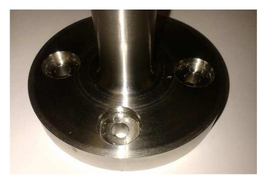
Figure 7.10: Fully Manufactured Cheek Plate
