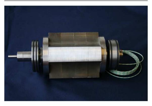
Figure 7.18: Fitted O'rings on the Bearing Cups
