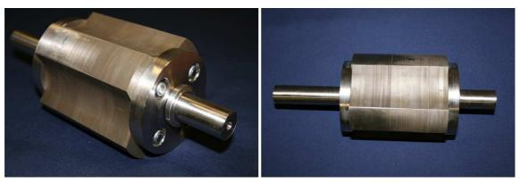
(a) Assembled Bearing Placing Ring
