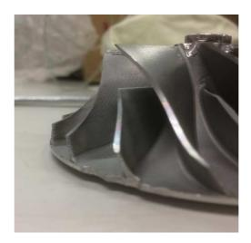
Figure 8.16: Evidence of Damage on the Compressor Wheel
