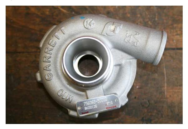
Figure 7.19: Volute of The Compressor Wheel, The Side Tube is Exhaust and the Middle One is the Inlet.
