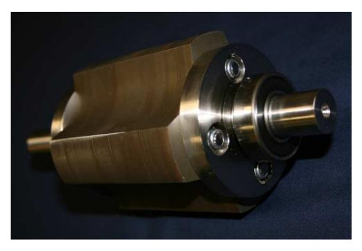
Figure 7.15: Bearing Assembled On the Rotor
