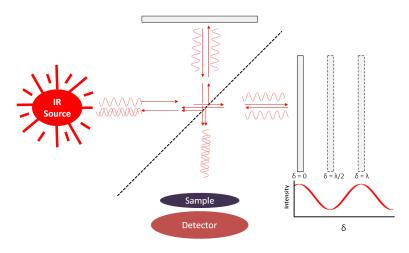
Figure 6.6: Principles of interferometry
