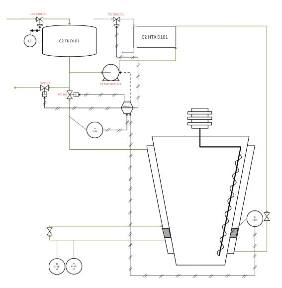
Figure A.11: Dryer D101 temperature control
