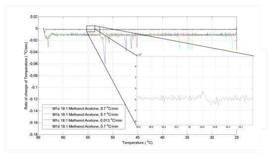
Figure 6.8: Rate of change of temperature vs. reactor contents temperature during crystallization experiments for system M1. Inset, blown up portion of the M1\_c experiment to show the location of crystallization.
