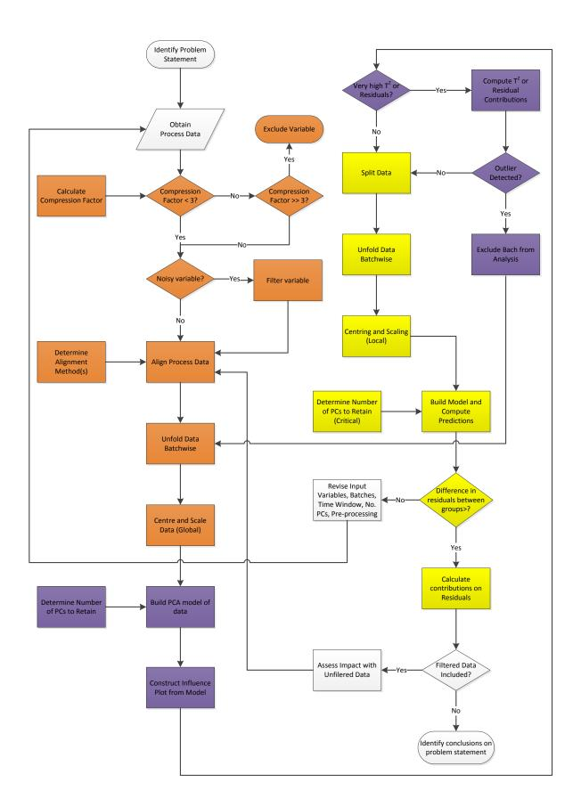
Figure 7.1: Overview of framework to extract multivariate information from batch process data (orange - pre-processing, blue - outlier detection, yellow - multivariate modelling, grey support the framework)
