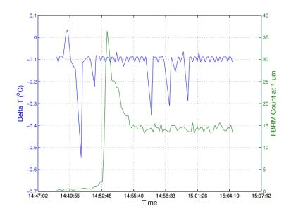
Figure 6.24: Differential temperature of experiment M1\_a around nucleation
