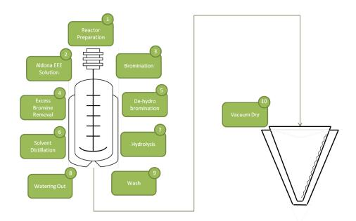
Figure 2.5: Aldona ethyl enol ether to Aldadiene manufacturing process
