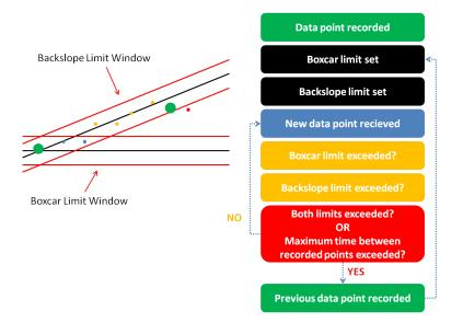
Figure 2.8: Process data compression algorithm
