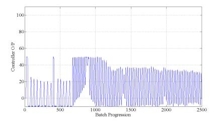
Figure 5.4: Temperature controller output with oscillations
