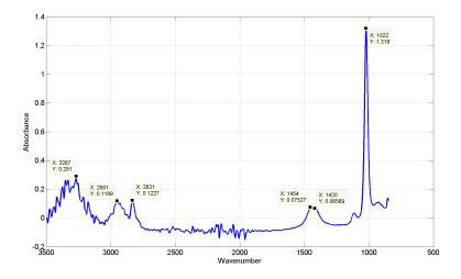
Figure 6.34: Raw ATR-FTIR spectra of methanol
