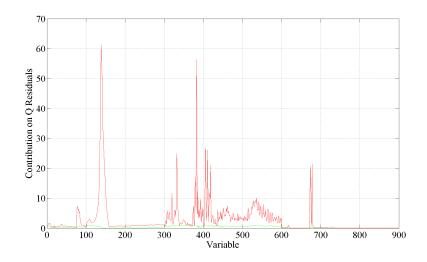
Figure 5.28: Contribution plot on the Q Residuals for the reactor data from the fast (green) and slow (red) drying batches
