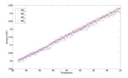
Figure 6.39: Temperature scores plot for PCA model on ATR-FTIR crystallization spectra on principal component 1
