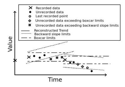
Figure 3.3: Boxcar backward slope compression.(Adapted from Watson et al. (1998))
