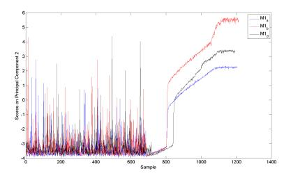
Figure 6.27: Scores plot on principal component 2 for NIR data from experiments M1
