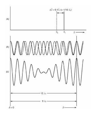
Figure 6.7: Example of how multiple wavenumbers produce information in the combined interefereogram (De Griffiths and Haseth, 2007).
