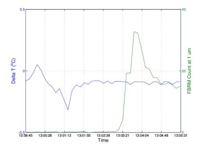
Figure 6.18: FBRM identification of nucleation in experiment M2\_a
