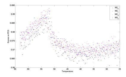
Figure 6.43: Temperature scores plot for PCA model on ATR-FTIR crystallization spectra on principal component 3
