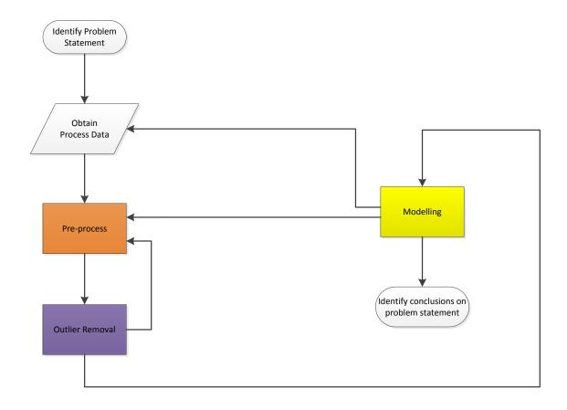
Figure 2.9: Overview of framework to extract multivariate information from batch process data (orange - pre-processing, blue - outlier detection, yellow - multivariate modelling, grey support the framework)
