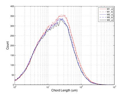
Figure 6.16: Effect of acetone concentration on Spironolactone chord length distribution
