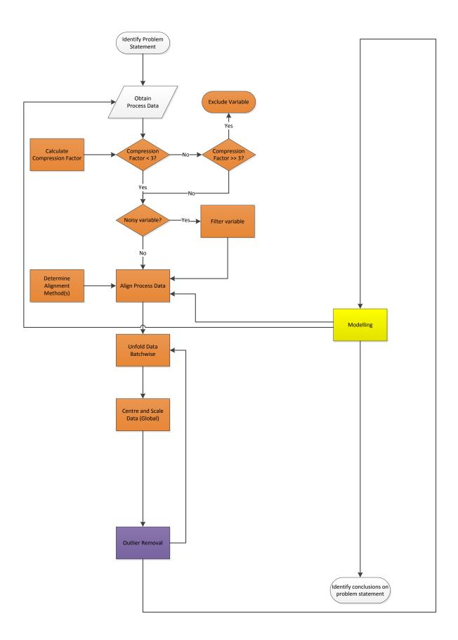
Figure 3.11: Overview of framework to extract multivariate information from batch process data highlighting (yellow) the pre-processing methods discussed in chapter 3
