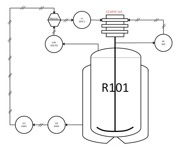
Figure A.6: Reactor R101 level control
