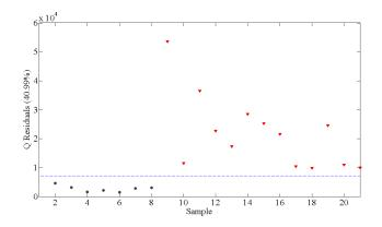
Figure 5.15: Q Residuals for the dryer data from the fast (black dots) and slow (red triangles) drying batches with the 95% confidence limit indicated
