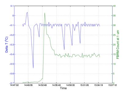
Figure 6.17: FBRM identification of nucleation in experiment M1\_a
