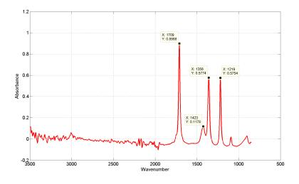
Figure 6.35: Raw ATR-FTIR spectra of acetone
