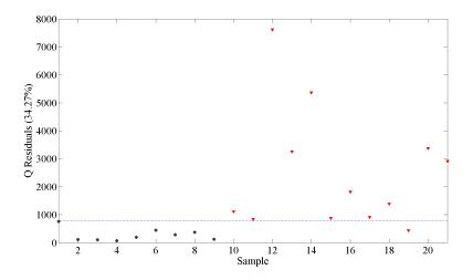
Figure 5.27: Q Residuals for the dryer data from the fast (black dots) and slow (red triangles) reactor batch data with the 95% confidence limit indicated
