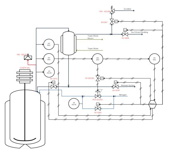
Figure A.4: Reactor R101 pressure control
