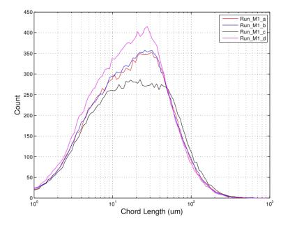
Figure 6.13: FBRM chord length distribution at end of experiments for group M1
