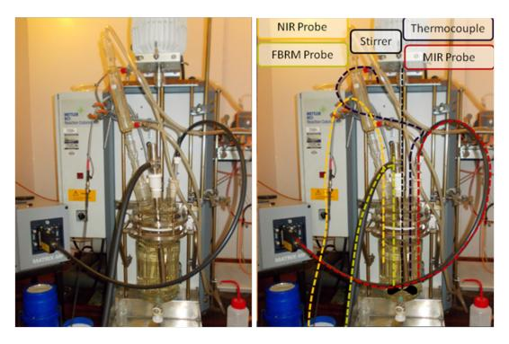
Figure 6.1: RC1 reactor with FBRM, ATR-FTIR, and NIR instruments
