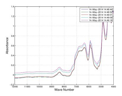
Figure 6.23: Raw NIR spectra of experiment M1\_a around nucleation
