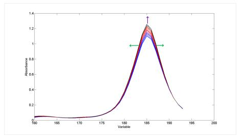
Figure 6.46: Baselined ATR-FTIR spectra M2\_b of methanol peak wave numbers showing peak broadening throughout crystallization (blue = start, red = middle, black = end of experiment)
