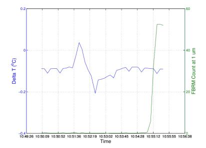
Figure 6.19: FBRM identification of nucleation in experiment M3\_a
