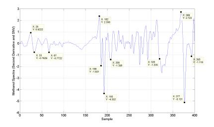
Figure 6.30: NIR spectra (second derivative and SNV) of methanol
