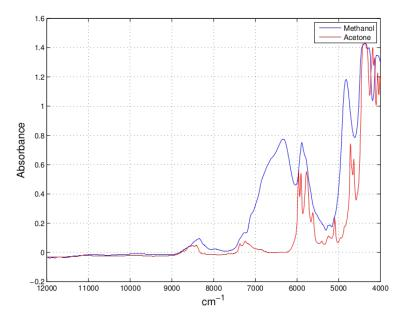
Figure 6.20: NIR spectra of pure methanol and pure acetone
