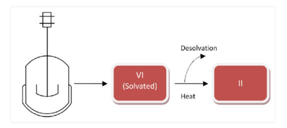
Figure 2.2: Spironolactone polymorph form II production through desolvation of the solvated form VI
