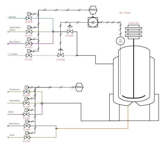
Figure A.3: Reactor R101 temperature control
