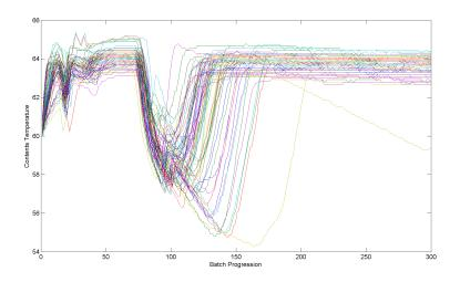
Figure 5.19: Pseudo aligned data for reactor contents temperature
