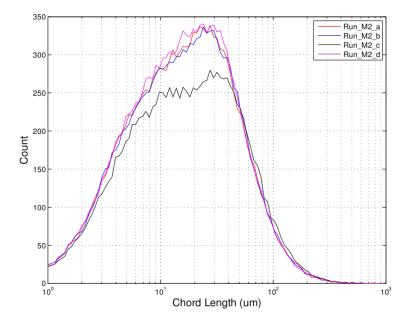
Figure 6.14: FBRM chord length distribution at end of experiments for group M2
