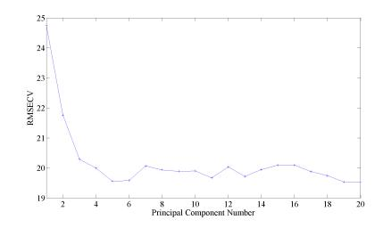
Figure 5.24: Root mean squared error for cross validation for dryer data
