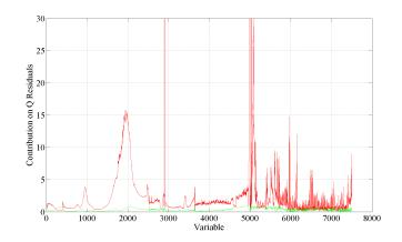
Figure 5.16: Contribution plot on the Q Residuals for the dryer data from the fast (black) and slow (red) drying batches
