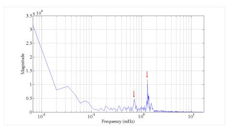
Figure 5.5: Single sided magnitude spectrum of the controller output signal (arrows indicating 0.7 mHz and 1.5 mHz)
