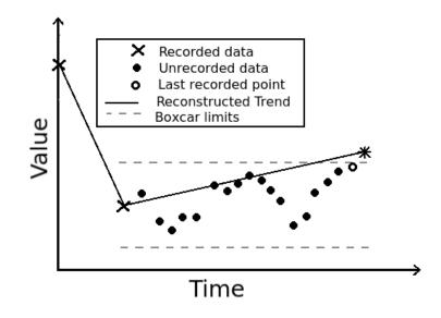
Figure 3.1: Boxcar compression. (Redrawn from Watson et al. (1998))
