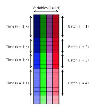
Figure 4.10: Unfolding X (IKxJ)
