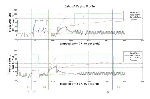
Figure 5.7: Misalignment in drying profiles of two batches due to process wait. A1 and B1 indicate the start of the second charge operation to the dryer for batch A and B respectively. A2 and B2 indicate the start of the second dry operation for batch A and B respectively. A3 and B3 indicate the end of the deodour operation for batch A and B respectively.
