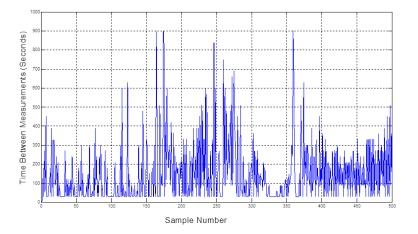
Figure 3.6: Sampling rate of compressed dryer temperature data following retrieval from data historian
