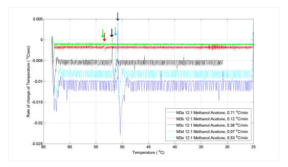
Figure 6.10: Rate of change of temperature vs. reactor contents temperature during crystallization experiments for system M3.
