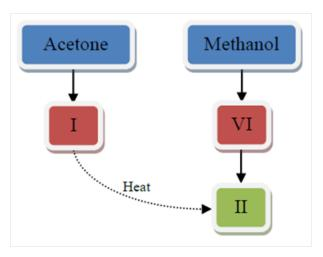
Figure 2.3: Spironolactone polymorphic form conversion routes from methanol and acetone crystallizations
