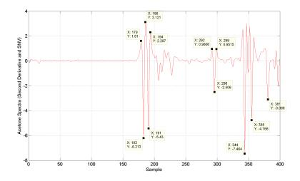
Figure 6.32: NIR spectra (second derivative and SNV) of acetone
