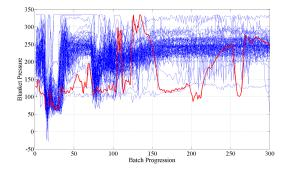
(a) Q residuals for batch 39 reactor data (b) Reactor blanket pressure data for batch 39
