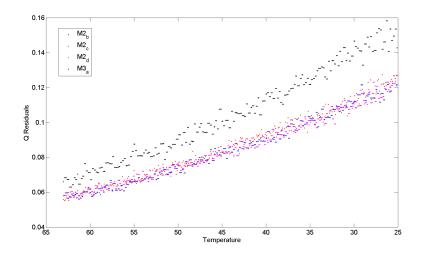
Figure 6.44: Temperature Q residuals plot for PCA model on ATR-FTIR crystallization spectra
