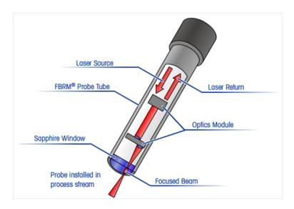
Figure 6.4: Diagram of FBRM probe operation
