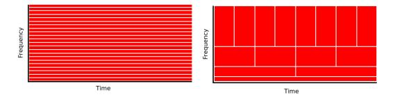
Figure 3.5: Resolution analysis representation of Discrete Fourier Transform (left) and Discrete Wavelet Transform (right). (Adapted from (Watson et al., 1998))
