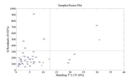
Figure 5.25: Influence plot of autoscaled reactor data unfolded in the batch direction with 95% confidence limits shown
