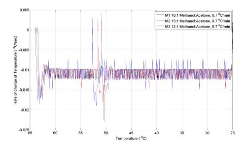
Figure 6.11: Rate of change of temperature vs. reactor contents temperature during crystallization experiments for system systems with varying quantities of acetone for the same cooling rate.
