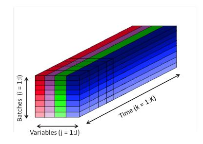
Figure 4.8: Three dimensional data matrix for batch process data
