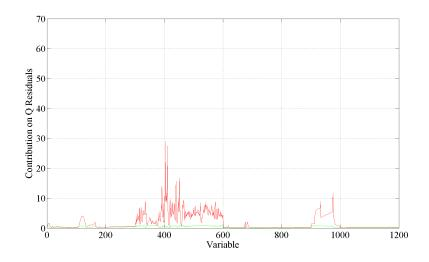
Figure 5.29: Contribution plot on the Q Residuals for the reactor data from the fast (green) and slow (red) drying batches for the data with feature alignment applied
