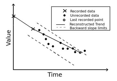
Figure 3.2: Backward slope compression. (Redrawn from Watson et al. (1998))
