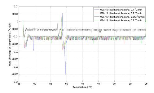
Figure 6.9: Rate of change of temperature vs. reactor contents temperature during crystallization experiments for system M2.
