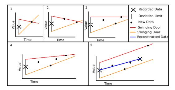
Figure 3.4: Swinging door compression algorithm
