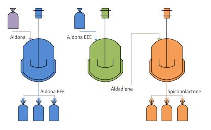
Figure 2.7: Simplified spironolactone manufacturing process schematic
