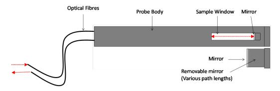
Figure 6.25: Transflectance NIR probe
