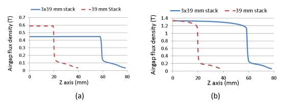
Figure 4-5: Representative flux density in the airgap. (a) 160%  $I_{pk}$ . (b) 400%  $I_{pk}$ .
