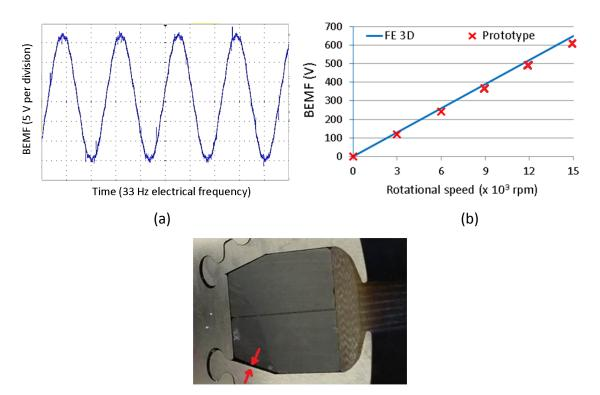
Figure 8-12: BEMF testing. (a) Prototype BEMF measurement at 33 Hz electrical frequency.
