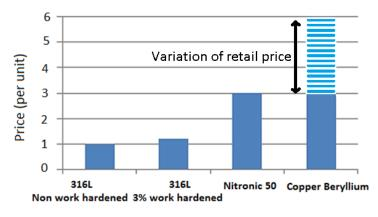
Figure 5-9: Price comparisons for the different rotor support materials.
