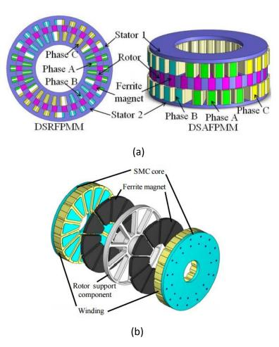
Figure 2-13: Innovative high torque density traction motor designs with ferrite magnets. (a) Dual stator topology [62]. (b) Axial flux motor with coreless rotor [63].
