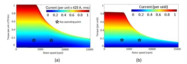
Figure 6-9 Distribution of current over torque-speed profile. (a) Fir tree based model. (b) Single piece model.
