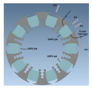
Figure 8-4: Demagnetization test configuration.
