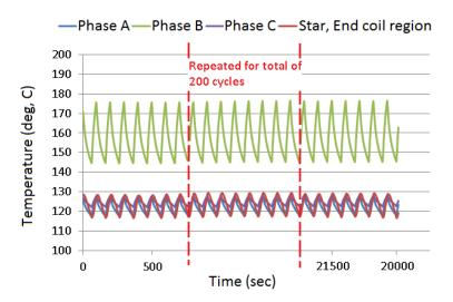
Figure 8-24: Evaluation of thermo-mechanical stability under cyclic loading.
