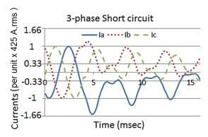
Figure 3-9: 3-phase short circuit currents.
