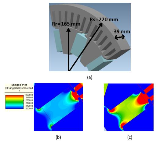
Figure III 80 kW first principle design using ceramic 8 magnets, and scaled diameter.
