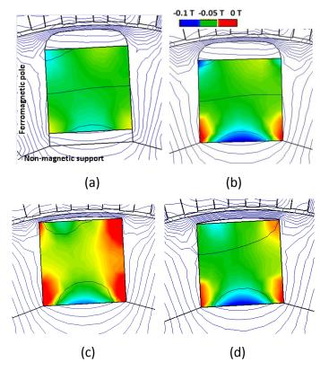
Figure 3-7: Demagnetization proximity. (a) 1 mm bridge, 4 mm and 3 mm top and bottom air voids. (b) 1 mm bridge, 4 mm top air void, no bottom air void. (c) 1 mm bridge, no air voids. (d) 2 mm bridge, no air voids.
