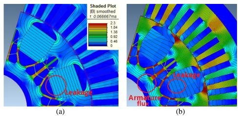
Figure 6-3 Flux lines and flux density in the single piece rotor design, and illustration of
