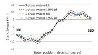
Figure VI Comparison of the static torque under 1-phase and 3-phase system excitations
