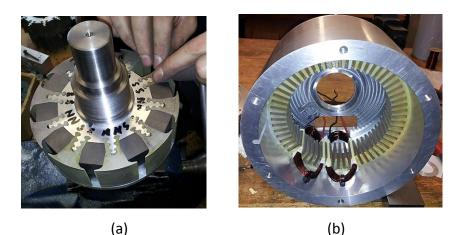
Figure 8-1: Simplified prototype motor. (a) Rotor and magnets, (b) Stator, coils and custom built housing without cooling.
