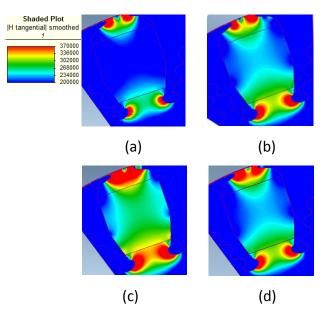
Figure V Comparison of the demagnetization behaviour under 1-phase and 3-phase system excitations, FE 2D, FB9B magnets. (a) 100%  $I_{pk}$  in 1-phase system. (b) 100%  $I_{pk}$  in 3- phase,  $I_b=I_c=-0.5 I_a$ . (c) 150%  $I_{pk}$  in 1-phase system. (d) 125%  $I_{pk}$  in 1-phase system.
