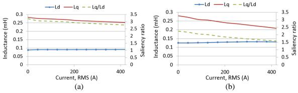
Figure 7-5: D and Q-inductance and saliency ratio vs. current. (a) Distributed winding. (b) Concentrated winding.
