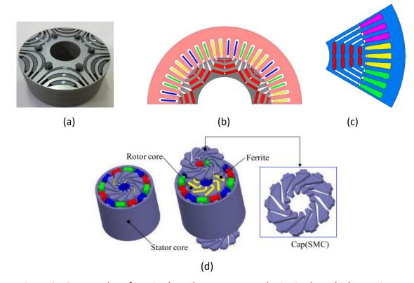
Figure 2-10: Examples of Ferrite-based IPM rotor topologies in the vehicle traction application. (a) U shape [40], (b) V shape [55], (c) U shape with horizontal magnets [23]. (d) LC shape [56].
