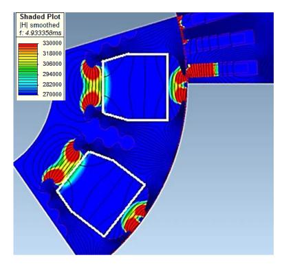
Figure 3-10: Field strength (A/m) distribution during 3-phase short circuit.
