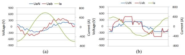
Figure 7-2: Voltage and current waveforms at 3 krpm rotor speed. (a) Distributed winding. (b) Concentrated winding.
