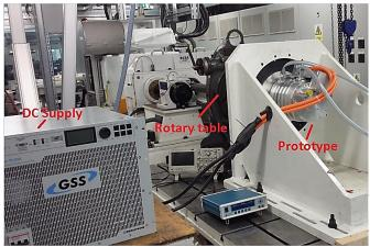
Figure 8-13: Static torque testing set up for the ferrite prototype motor.
