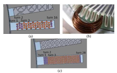
Figure 7-8 The layout of turns and parallel wires in the distributed winding design. (a) Organized layout, STAR. (b) A sample of manufactured coil. (c) Organized layout, DELTA.
