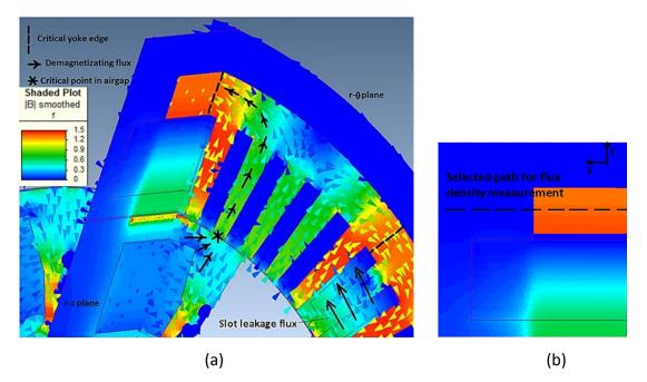
Figure 4-3: 3D flux vector and flux density distribution in 39 mm stack model, under 160% I<sub>pk</sub>.
