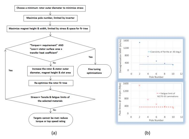
Figure 3-3: (a) Design optimization algorithm of the spoke type design. (b) Influence of the number of poles on the demagnetization and rotor stress.
