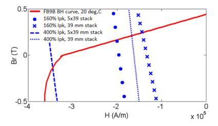
Figure 4-7: Magnet BH curve and load lines for scenarios with different short circuit currents (accounting for saturation) and stack lengths.
