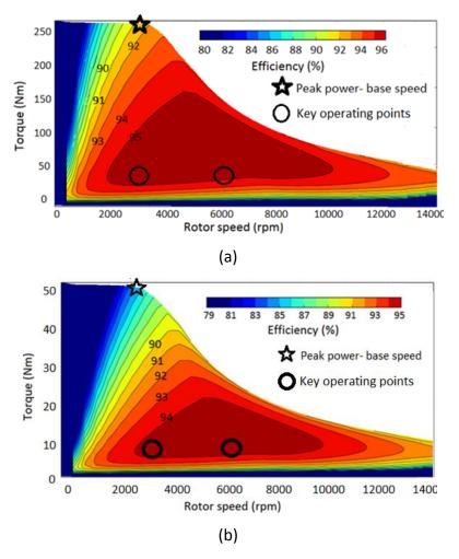
Figure IV Comparison of peak torque-speed performance and efficiency map for FB9B ferrite designs with different stack lengths. (a) 195 mm stack length. (b) 39 mm stack length.
