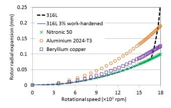
Figure 5-3: Comparison of rotor radial expansions for various rotor support materials.
