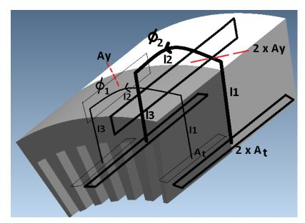
Figure II Illustration of the variation of stator laminations reluctance by varying (halving) the stack length.
