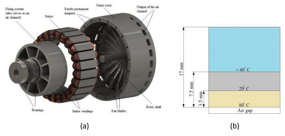
Figure 2-15: A 50 kW surface mounted ferrite design, and the required temperature levels in the magnets to avoid demagnetization [67]. (a) Topology. (b) Required temperature levels.
