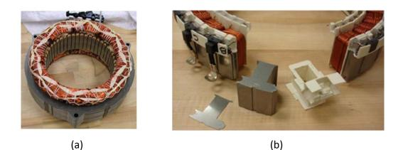
Figure 2-19: Comparison of a non-modular vs. modular stator. (a) Prius 2010 [36]. (b) Honda Accord 2005 [37].
