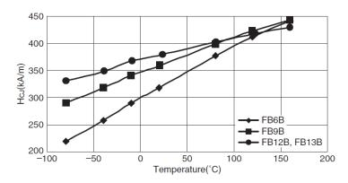
Figure 2-14: Coercivity and its temperature dependency for some typical high grade ferrite magnets, [64].
