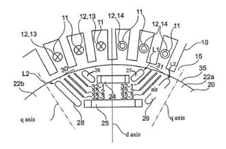
Figure 2-6: An illustration of BMW i3 traction motor rotor design [45].
