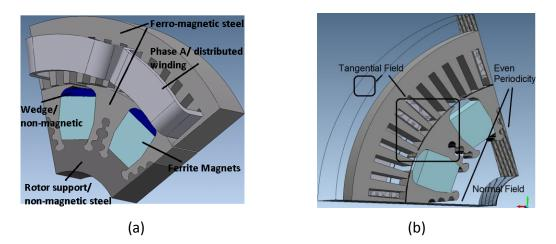
Figure 4-1: (a) 3D model of the reference motor design, with one-tenth of the original length. (b) Boundary conditions.
