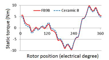
Figure 4-10: Comparison of the static torque for the 39 mm stack length designs using FB9B and Ceramic 8 magnet grades.
