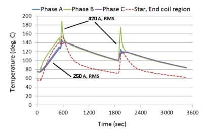
Figure 8-23: Temperature rise vs. continuous and peak current.
