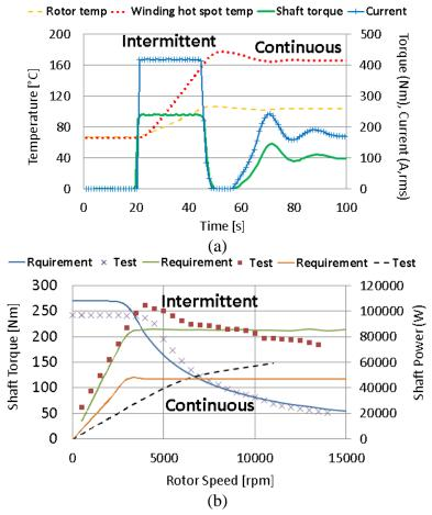
Figure 8-26: Intermittent and continuous performance of the HSFM prototype under 400 V DC link voltage. (a) At 3000 rpm. (b) Test vs. requirement performance for the entire speed
