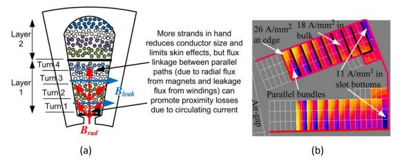
Figure 2-20: Illustration of AC winding losses, [96]. (a) Flux leakage in the slot. (b) Increased current densities due to proximity effects.
