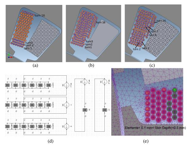
Figure 7-6: The layout of turns and parallel wires in the concentrated winding design, circuit and mesh view. (a) Organized layout with low fill factor. (b) Random layout with high fill factor, optimistic. (c) Random layout with high fill factor, pessmistic.(d) External circuit driving the 3-phase coils, and parallel strands.(e) Mesh view.
