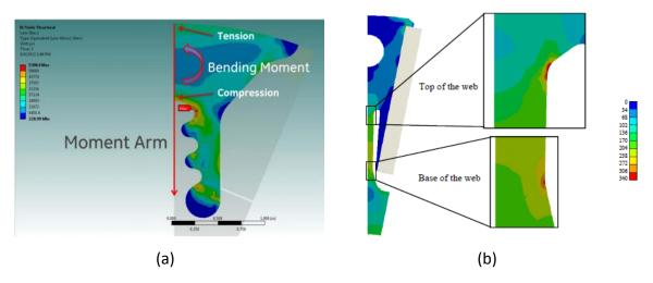
Figure 2-18: Illustration of the rotor peak stress distribution during high speed operation.(a) Spoke type with fir tree design, 14,000 rpm top speed [34]. (b) Spoke type with single piece rotor, 11,000 rpm to speed [35].
