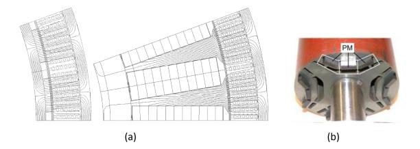
Fig 2-8: Examples of high performance ferrite based machines designs. a) Wind generator comparing NdFeB to ferrite based designs, [53]; b) A synchronous reluctance Ferrite assisted for industrial application [54].
