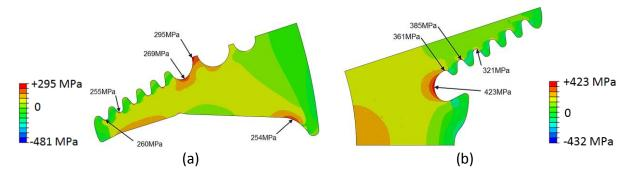
Figure 3-12: Stress distributions at 15 krpm, initial fir-tree design. (a) Rotor pole. (b) Rotor support.
