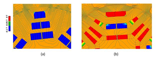
Figure 3-1: Demagnetization proximity, PMASynR U-shape designs with ferrite magnets. (a) 8-pole design. (b) 4-pole design.
