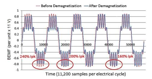
Figure 8-5: BEMF before and after negative d-axis current injections, at 33 Hz electrical frequency.
