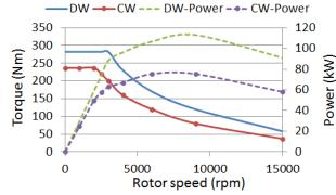
Figure 7-4: Torque vs. speed for distributed against concentrated winding.
