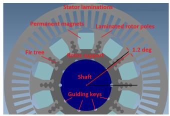
Figure 5-1: Spoke type ferrite motor design, 2D topology.
