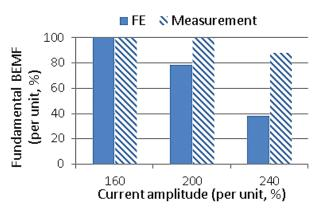
Figure 8-7: Loss of BEMF fundamental component due to demagnetization; prototype measurement compared against 2D FE.
