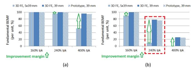
Figure 8-9: Loss of BEMF fundamental component due to demagnetization. (a) FB9B magnets. (b) Ceramic 8 magnets.
