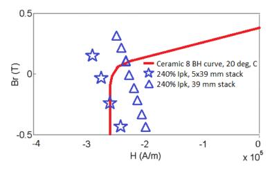
Figure 4-9: Demagnetization assessment using the proposed lumped circuit model,
