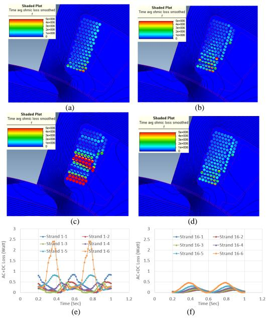
Figure 7-7 Winding AC + DC loss distribution, 2D FE. (a) Organized layout. (b) Random layout, optimistic. (d) Random layout, Pessimistic. (d) Random layout, optimistic, Aluminium wires.(e) Loss per strand in turn 1, organized lay-out, Copper. (f) Loss per strand in turn 16, organized lay-out, Copper.
