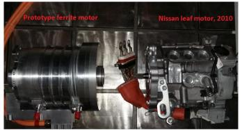
Figure 8-11: Comparison of the full size prototype ferrite motor with Nissan leaf motor.
