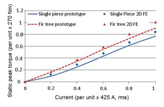
Figure 8-19: Static torque vs. current; comparison of single piece and fir-tree based rotor designs.
