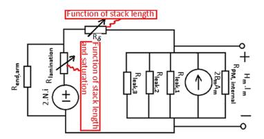
Figure 4-6: Magnetic lump circuit for 3D modelling of demagnetization.
