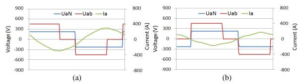
Figure 7-3: Voltage and current waveforms at 15 krotor speed. (a) Distributed winding. (b) Concentrated winding.
