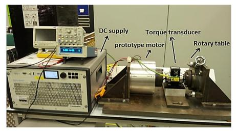
Figure 8-2: Prototype test set-up.
