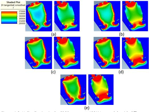
Figure 4-2: H distribution in the FB9B magnets, 400% I<sub>pk</sub>, models with different stack lengths.
