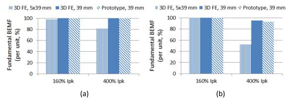
Figure 8-21: Loss of BEMF fundamental component due to demagnetization. (a) Single piece rotor model. (b) Fir tree based rotor model
