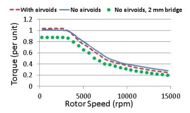
Figure 3-8: Torque-speed comparison for designs with/ without air voids and different bridge thicknesses (the effect of demagnetization on the torque is excluded).
