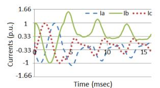
Figure 6-5: 3-phase short circuit currents for the single piece design.
