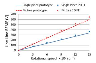
Figure 8-18: BEMF vs. rotor speed; comparison of the single piece and fir-tree based rotor
