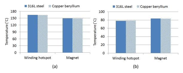
Figure 5-8: Effect of rotor support material on the winding and magnet temperature. (a) Continuous operation at 60 kW, 10 krpm. (b) Continuous operation at 10 kW, 6 krpm.
