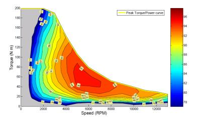
Figure 2-2: Prius 2010, Motor-Inverter combined efficiency, [36].
