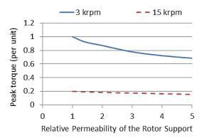
Figure 5-5: Peak torque capability at base and top speed vs. rotor support permeability.
