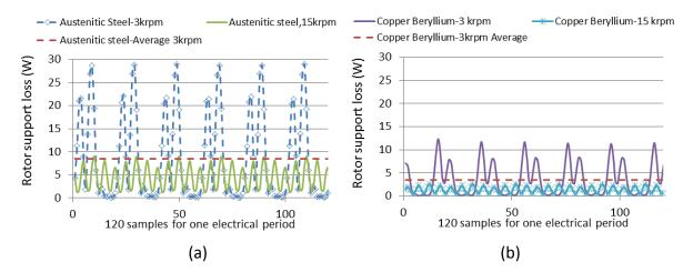
Figure 5-6: Rotor support losses for the peak power operating points at 3 krpm and 15 krpm rotor speeds. (a) Austenitic steel rotor support. (b) Copper beryllium rotor support.
