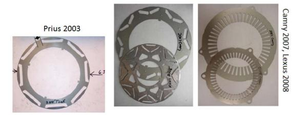
Figure 2-1: Rotor topology in different Toyota EV designs, [17], [36].
