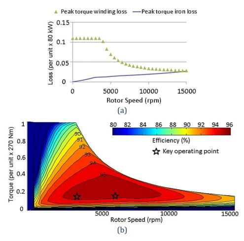
Figure 3-6: Loss and efficiency map of the proposed spoke design. (a) Winding and iron loss for peak power operation. (b) Efficiency map.
