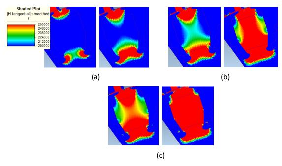
Figure 4-8: Field strength distribution in the Ceramic 8 magnets, for designs with 195 mm stack length (right column), and 39 mm stack length (left column), and under negative d-axis currents with different amplitudes. (a) 160% I<sub>pk</sub>. (b) 240% I<sub>pk</sub>. (c) 400% I<sub>pk</sub>. All results correspond to middle stack faces.
