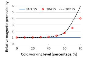
Figure 5-4: Change of magnetic permeability vs. work hardening [112].
