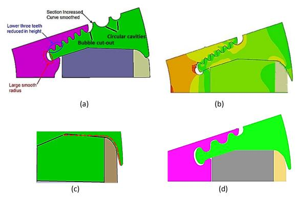
Figure 3-11: Evolution of the rotor structural designs. (a) Initial design. (b) Top cavities removed. (c) Parallel vs. tapered face magnets. (d) Number of teeth reduced.
