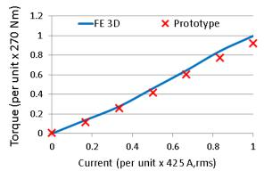
Figure 8-14: Static peak torque against current; prototype testing vs. 3D FE simulation.
