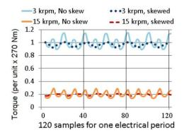
Figure 3-5: Peak transient torque waveforms at base and top speed, with and without skew.
