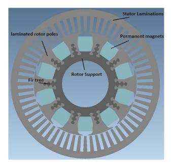
Figure 3-4: A cross section of the optimized spoke type design.
