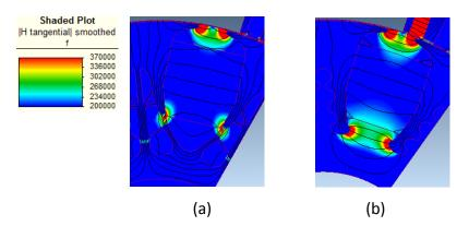
Figure 6-6: Demagnetization risk assessment (H distribution) under 160% lpk in negative daxis location and FB9B magnets. (a) Single piece trial design. (b) Fir-tree based design.
