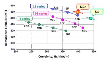
Figure 2-9 Comparison of different top grades of Ferrite magnets [20].
