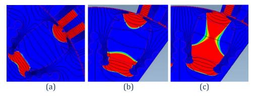
Figure 8-6: 2D FE predicted demagnetization (H) with different current amplitudes applied in negative d-axis. (a) 160% lpk. (b) 200% lpk. (c) 240% lpk.
