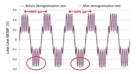
Figure 8-20: BEMF prior and after the demagnetization test, single piece design, at 10 rpm.
