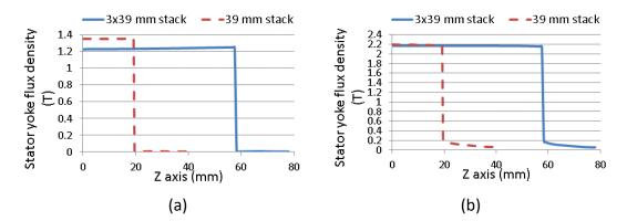
Figure 4-4: Representative flux density in the stator. (a) 160%  $I_{pk}$ . (b) 400%  $I_{pk}$ .
