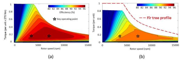
Figure 6-8: Efficiency map for complete torque-speed profile. (a) Fir tree based model. (b) Single piece model.
