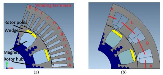
Figure 7-1: Schematics of high speed ferrite motor. (a) Distributed winding, Motor stack length=195 mm. (b) Concentrated winding, Motor stack length=255 mm.
