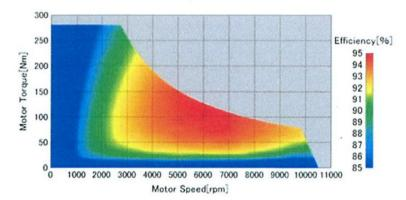
Figure 2-4: Efficiency map of the Leaf power train including motor, inverter and AC cables. [38].
