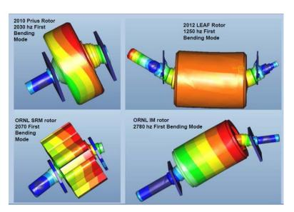
Figure 2-17: Illustration of critical speed bending at high speeds [79].
