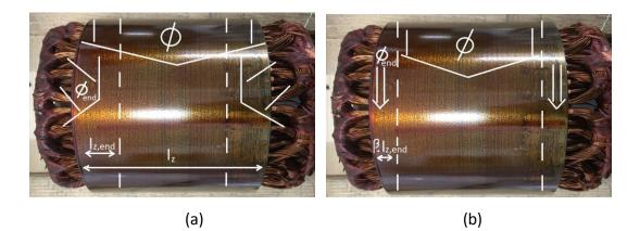
Figure I: Illustration of the reduced effective surface area for the demagnetizing field/ flux. (a) Actual model. (b) Equivalent model.
