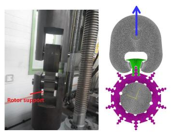
Figure 8-16: Rotor fatigue testing under cyclic loading.
