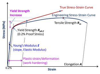
Figure 5-2: Illustration of tensile stress-strain curve.
