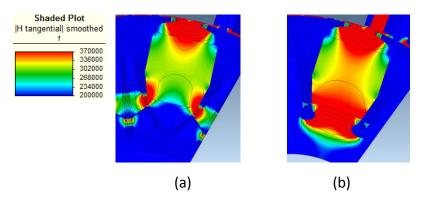
Figure 6-7: Demagnetization risk assessment (H distribution) under 400% lpk in negative daxis location and FB9B magnets. (a) Single piece trial design. (b) Fir-tree based design.
