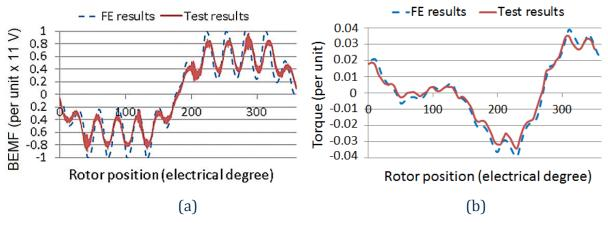
Figure 8-3: Motorette performance, comparison between measured and FE calculations. (a) BEMF at 33 Hz electrical frequency. (b) Static torque vs. different rotor angles.
