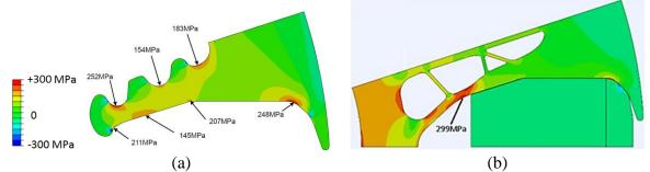
Figure 6-2: Stress distributions at 15 krpm for fir-tree and single piece rotor design. (a) Fir tree based rotor pole. (b) Single piece rotor.
