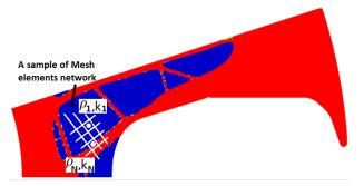
Figure VII Illustration of the stress-constrained mass minimization technique, employed for optimizing the single piece rotor design topology.
