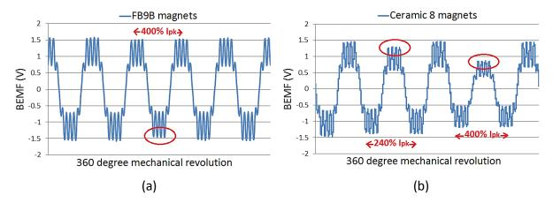
Figure 8-8: BEMF waveforms after the demagnetization test. (a) FB9B. (b) Ceramic 8.
