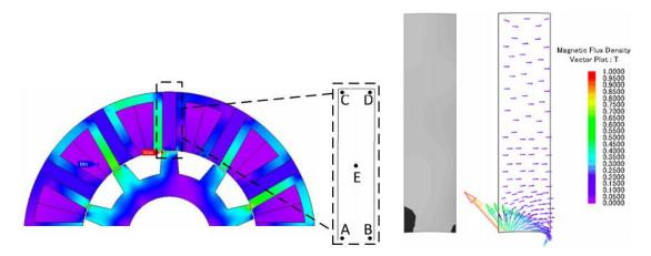
Figure 2-16: Illustration of a partial demagnetization in a flux switching ferrite based traction motor, [72].
