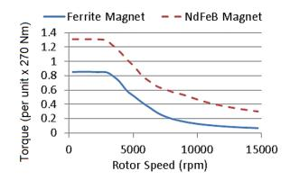
Figure 3-2: Torque-speed performance of 8-pole PMAsynR design with ferrite and NdFeB magnets.
