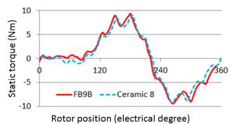
Figure 8-10: Comparison of static torque test results for 39 mm stack length design using
