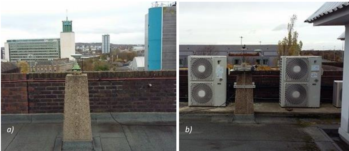
Figure 5.2: a) DRMB antenna and concrete pillar mount, looking South. b) DRMS antenna, concrete pillar and moving platform mount, looking North.
