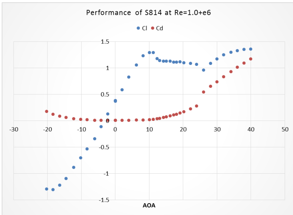
Figure 3-3 Experimental result of the performance of S814 at Re=1+e6 (Janiszewska et al. , 1996)
