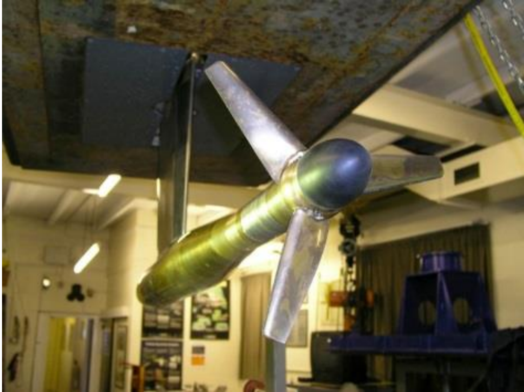
Figure 3-2 Scaled tidal turbine model mounted on the dynamometer of Emerson Cavitation Tunnel
