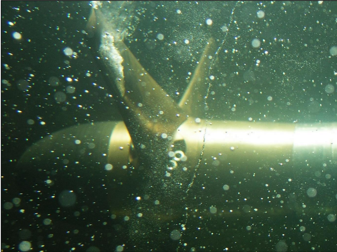
Figure 2-30 Cavitation observed at shallow shaft immersion and designed stream speed (Wang et al. , 2007a)
