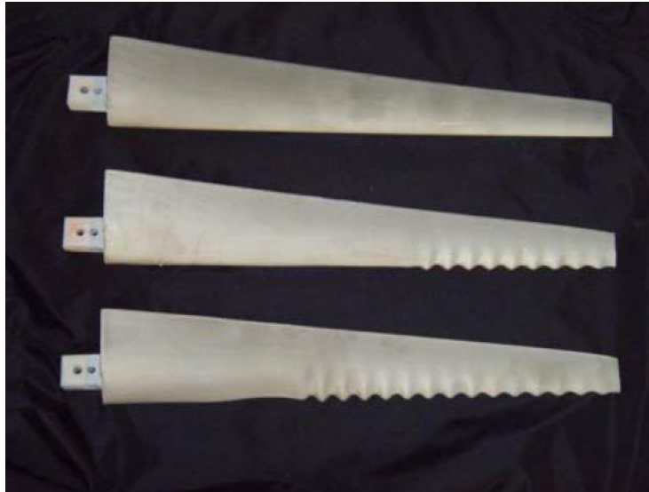
Figure 2-23 Tidal turbine blades (Top: Control Blade. Middle: 1/3 Tubercled. Bottom: 2/3 Tubercled) (Gruber et al. , 2011)
