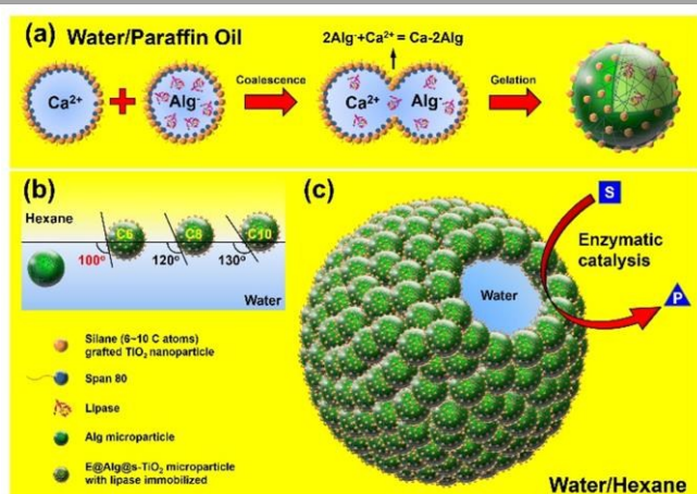
Scheme 1. Schematic representation of enzyme-immobilized surface-active Alg microparticles stabilizing W/O Pickering emulsions for interfacial biocatalysis: (a) Preparation of E@Alg@s- \text{TiO}_2 microparticles through Alg gelation via coalescence of water-in-paraffin oil emulsions, (b) wettability adjustment of E@Alg@s- \text{TiO}_2 microparticles at the water-hexane interface by chain length of grafted silane, (c) enzymatic catalysis at the interface of water-in-hexane Pickering emulsion. Substrate S, product P.
