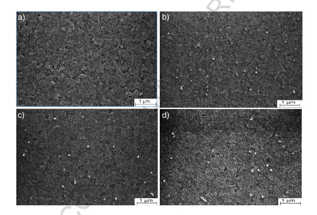
Fig. 5: SEM images of a) a control sample that has received a seed layer and has been dipped into the growth solution for one minute, and samples containing seed layers that were heated in a commercial microwave at 100% power for b) 20 s, c) 40 s and d) 60 s. In each case the ITO is clearly visible whilst images in c) and d) show the very early stages of nanowire growth. Early stages of crystallite growth also appear as white protrusions.
