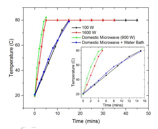
Fig. 4: Temperature profiles of the different heating methods used for growth of the ZnO nanorods. The methods consisted of a scientifc grade microwave with heating at 100 W (black data) and 1600 W (red data), and a domestic microwave with (blue data) and without (green data) a water bath. The inset shows an enlarged view of the temperature profiles during only the ramping step.
