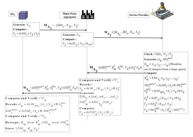
Fig. 2. Authenticated initialization and refilling process.
