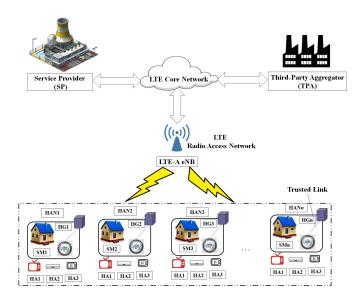
Fig. 1. System model for smart metering infrastructure.
