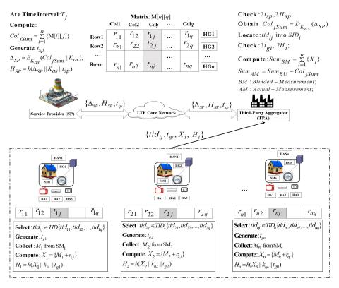
Fig. 4. Proposed computationally efficient and lightweight data aggregation scheme for demand-response management in smart grids.
