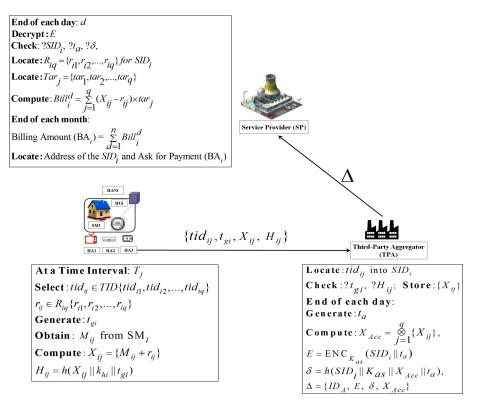
Fig. 3. Proposed computationally efficient and lightweight data aggregation scheme for secure dynamic pricing-based billing process in smart grids.
