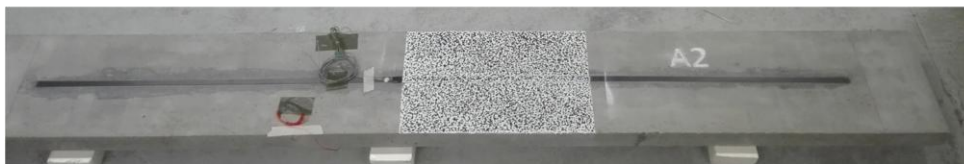
Test 2: RC slab with FRP strip; A_f = 37.5 \text{ mm}^2
