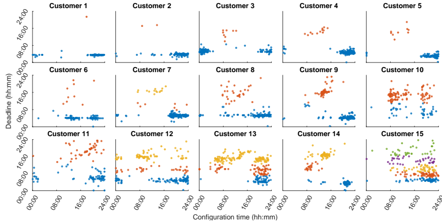
Figure 2.2: Clusters of deadlines from Stage I in the customer flexibility profiles for dishwasher. Each cluster is shown in a different color.
