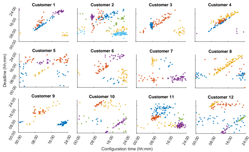
Figure 2.7: Bivariate Gaussian mixture fits and the resulting MAP clusters for washing machine flexible usage (in distinct symbols and colors; contour plots omitted for clarity).
