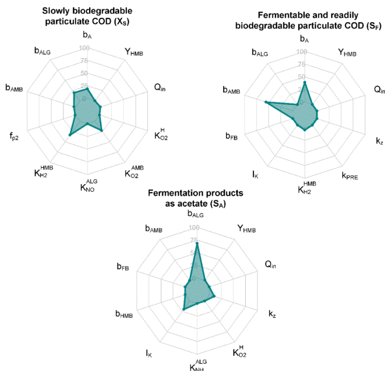
Figure 3. Ten most significant parameters influencing the variability of slowly biodegradable particulate COD, fermentable and readily biodegradable soluble COD, and fermentation products as acetate in
