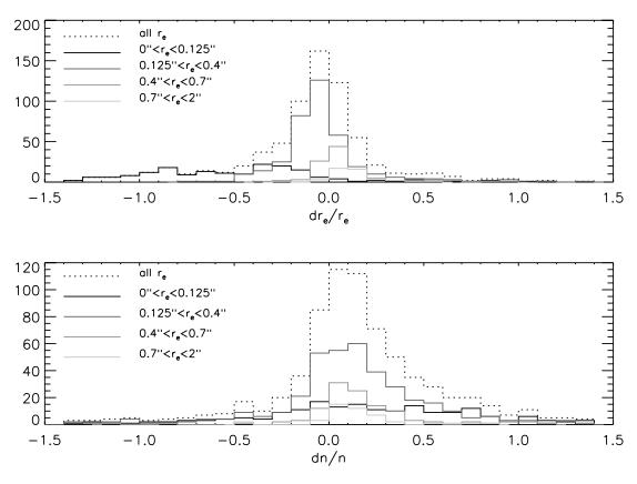
Fig. 4.—Reliability of the structural parameter estimation using different PSFs. *Top:* Relative difference between the circularized sizes estimated in the  $K_s$  using a PSF with an FWHM equal to the median value of the different PSFs (PSF1) and the size measured using a PSF with an FWHM 2  $\sigma$  times larger than the median (PSF2):  $dr_e/r_e = 2(r_{e,PSF2} - r_{e,PSF1})/(r_{e,PSF2} + r_{e,PSF1})$ . [See the electronic edition of the Journal for a color version of this figure.]
