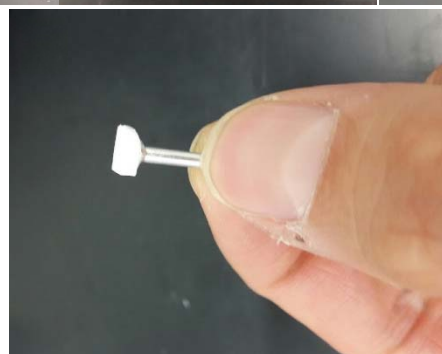
614 Figure S11: Trimming procedure to obtain samples before sectioning into thin (3 \mu m) samples using a microtome. a) IM 615 tablet attached to the entry section (i.e., gate). b) Tablet cut in half with a razor blade. f) Trimming of the tablet and mounting 616 on an aluminum pin. g) Final sample obtained before cryosectioning.
