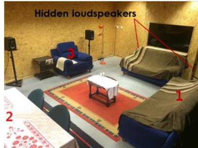
Figure 2 – The mock-up living room with hidden loudspeakers indicated next to the mock-up window.
