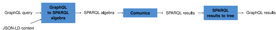
Fig. 1: Flow of GraphQL queries and JSON-LD contexts to SPARQL algebra, to SPARQL results, and to a tree shape.
