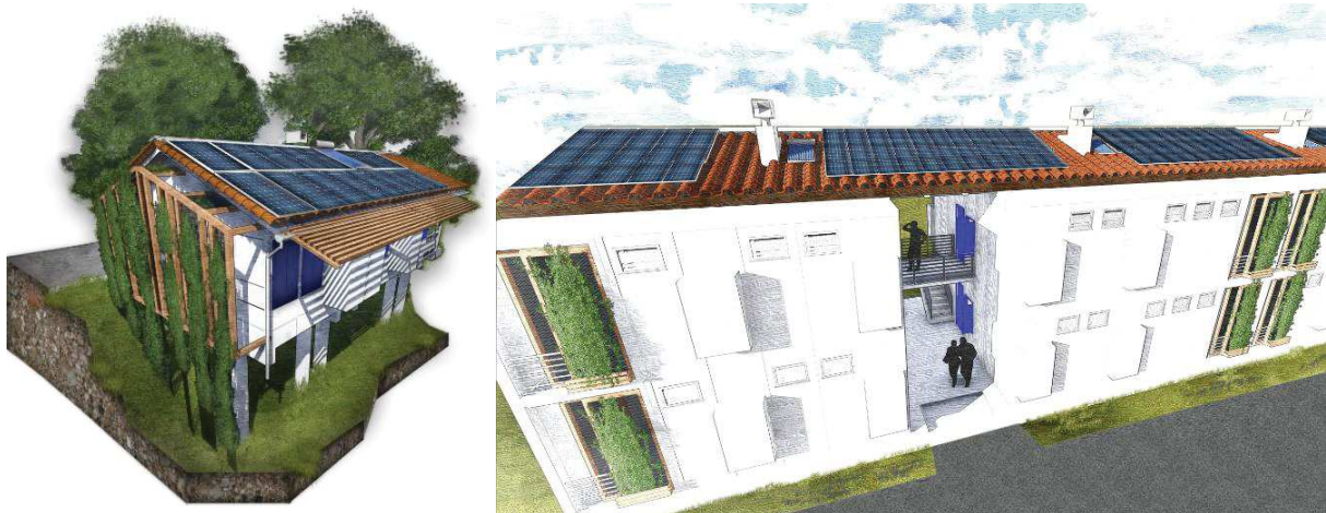
Figure 10-11. Transformation of Las Terrazas housing looking for better solar protections and incorporate renewable energy technology. Source: students of last course 2018.
