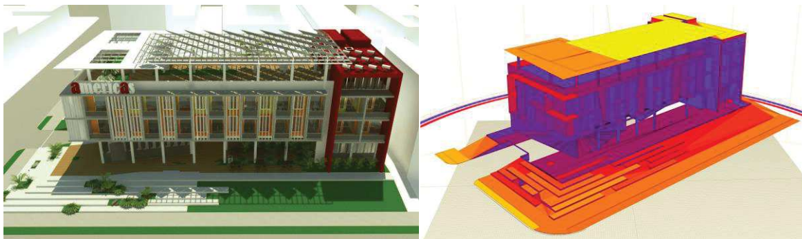
Figure 6-7. A student's design that cover the terrace snack bar with a photovoltaic roof as well as it was simulated the envelope design performance. Source: students of last course 2017.
