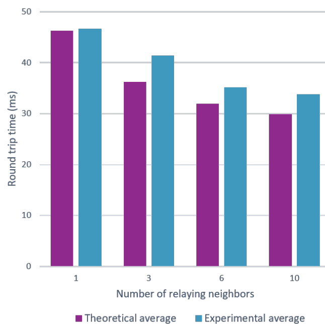
Figure 12. Two hop communication measurements with a varying amount of neighbors.
