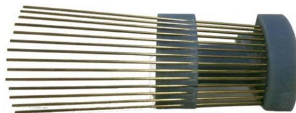
Figure 7. High precision, 3D printed, insertion guide to simulate forepoling in small scale physical models (from Le and Taylor)
