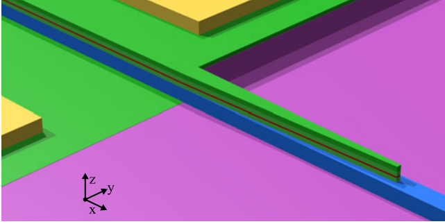
Fig. 5. Visualization of the taper, showing a waveguide (blue) on top of BCB (pink) being tapered into the modulator.
