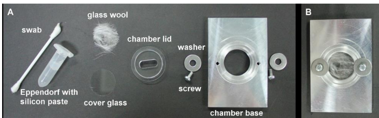
Figure 2: Imaging chamber assembly. A) The imaging chamber components. B) Assembled imaging chamber.
