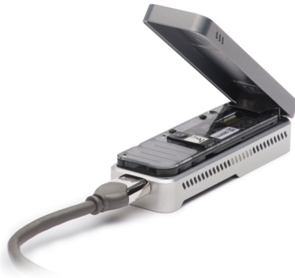
Figure 1.7: The Oxford Nanopore MinION, a thumb drive sequencer.
