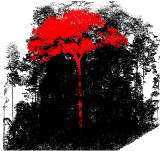
FIGURE 1 Using treeseq to extract a tree-level point cloud (red) from a larger-area point cloud (black) ( 35 \times 25 \times 47 m L \times W \times H) acquired from terrestrial laser scanning in tropical forest in Nouragues Nature Reserve, French Guiana
