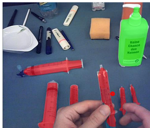
Figure 3: Detection of the two objects syringe and bottle by the cGOM algorithm. The detected objects are marked with masks, coloured according to the object class. Their positions in the image are then compared with the corresponding gaze point coordinate (red ring).
