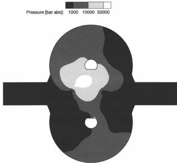
Figure 3.9: Pressure distribution on the unrefined grid of 4196 cells
