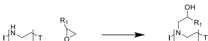
Scheme 8. Ring opening of an epoxide with L-PEI yielding the corresponding tertiary amine.
