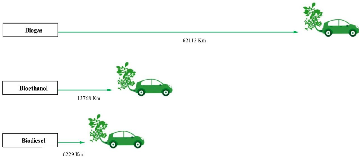
Fig. 3. The distance a car can travel using various biofuels (average fuel consumption was assumed to be 10 L/100km)
