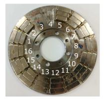
**Figure 7.** Faulty rotor disc with partial demagnetization: the complete third and fourth magnet, and a part of the eighth magnet are removed.
