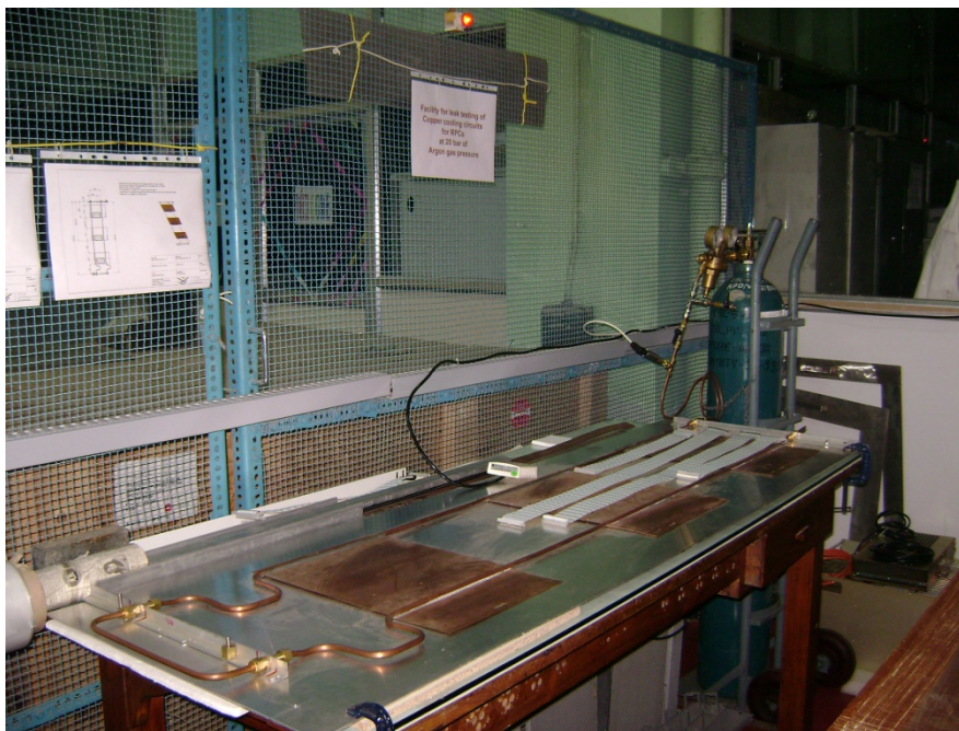
Figure 3. Cu cooling assembly for a typical RE4/3 RPC, under leak test after fabrication.
