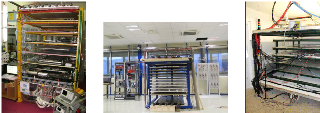
Figure 5. Cosmic hodoscopes at Mumbai (left), CERN (middle) and Ghent (right) assembly sites.
