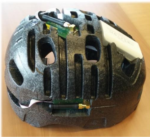
Figure 1. The PDE-Helmet. The locations of the antennas inside the helmet are shown on top. The interior of the helmet showing the padding in black, the folded stub antennas with receiver nodes in green-black-gold, and the battery in white, are shown on the bottom left. The device in its final form-factor is shown on the bottom right.
