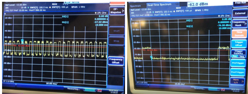
Fig. 4. The background traffic in the time domain: the traffic on channel 1, shown on the left side, has on average a 2 ms period and a duty cycle of roughly 50%; the channel 2 traffic, shown on the right side, has on average a 70 ms period and occupies the channel for about 13% of the time.
