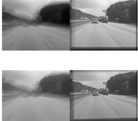
Fig. 4. Example of video stabilization performance of the proposed method (top) vs. a pixel-based method (bottom) [1], [22]. We compare the mean of the raw (left) vs. the corrected (right) frames for a random group of ca. 10 luminance frames.
