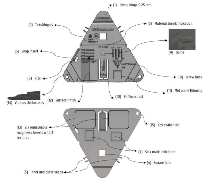
Figure 4: Features of the dEEEterminator.
