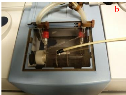
Figure 3.8. Gas analyzing instrumentation with (a) FT-IR, (b) cell in FT-IR (c) gas cell
