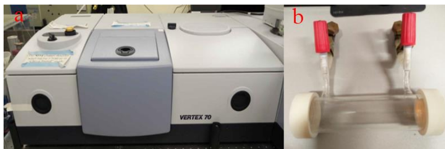
Figure 3.31 Gas analyzing instrumentation with (a) FT-IR, (b) gas cell
