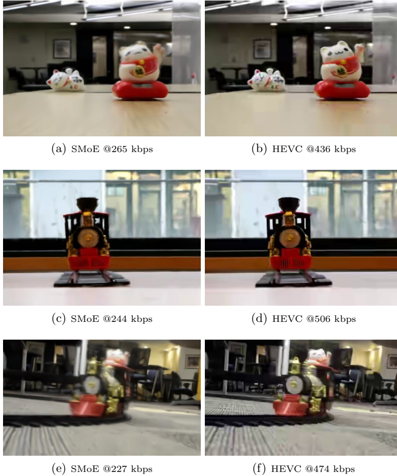
Figure 8. Subjective comparison of SMoE (left) vs. MV-HEVC (right) used in this work for datasets cats (top), train1 (middle) and train2 (bottom) both at 33dB, 32dB and 30dB PSNR respectively. However, the bitrate savings for this example are in the range of 50% for SMoE.
