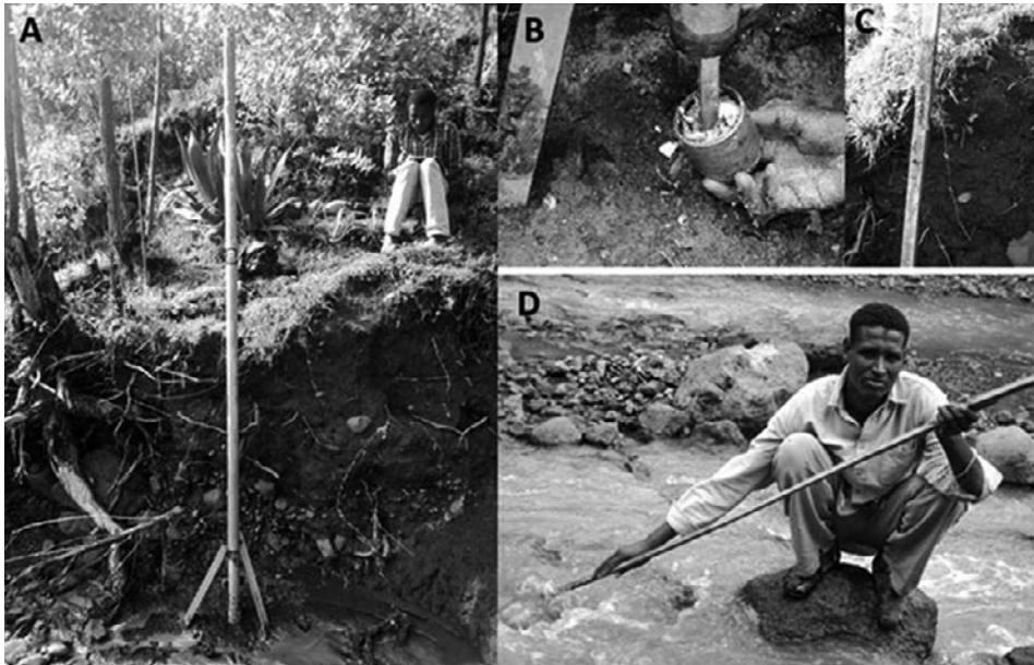
Figure 4: Crest stage gauge (A), sawdust being placed in the bowl of the lower cap before and after measuring peak stage (B), remnants of sawdust on wood staff indicating the highest peak stage of the flood (C), and wood staff being cleaned for the next flood (D).
