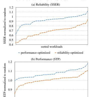
Fig. 6: System soft error rate (a) and system throughput (b) for reliability- and performance-optimized scheduling normalized to random scheduling for all four-program workloads on an HCMP with 2 big cores and 2 small cores.
