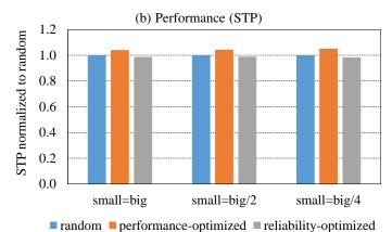
Fig. 14: SSER (a) and STP (b) of four-program workloads on a 2B2S system with decreasing L1 cache size for the small cores.
