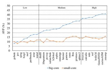
Fig. 1: AVF for the SPEC CPU2006 benchmarks on a big out-oforder and a small in-order cores. The benchmarks are sorted by their AVF on the big core.
