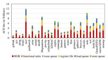
Fig. 5: ABC stacks for the out-of-order core.
