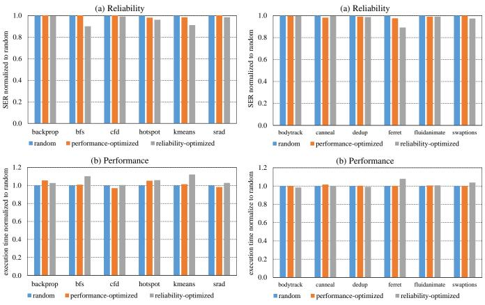
Fig. 11: Reliability (a) and performance (b) for the Rodinia benchmarks on a 2B2S system.
