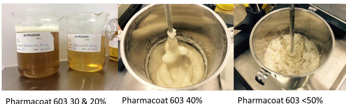
Figure 1. Pictures of Pharmacoat 603 binder liquids at different concentrations (% m/m). Right picture: state before obtaining a binder concentration of 50%.
