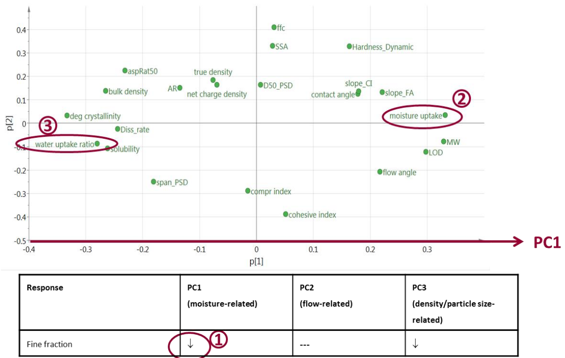
Figure 10. Example for the link between underlying filler properties, principle components and the response "fine fraction of granules" (important information in the PCA loading plot is highlighted in red)
