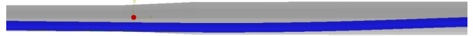
FIGURE 10: Illustration of the contact between the yarn and the analytical rigid body at t = 6.5 ms . The dot is located at an axial coordinate of 0.036 m .
