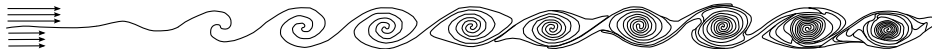
Figure 2: Kelvin-Helmholtz Instability (KHI) following a perturbation of the shear layer dividing two flows of different velocity leading to the formation of billows, spirals and elliptical vortices, poetically referred to as ‘cat eyes’.
