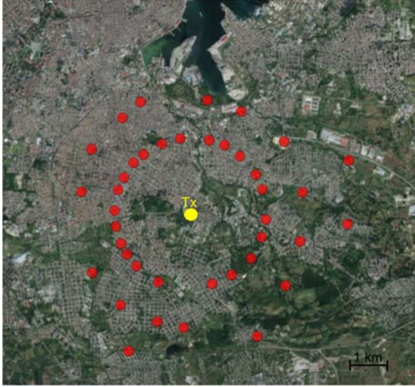
Fig. 3. Broadcast transmitter (TX yellow circle) and 40 measurement locations (red circles).
