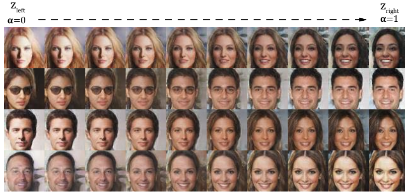
Figure 11: Linear interpolation of latent vector. Each row is the interpolation from left latent vector z_{left} to right latent vector z_{right} . e.g. (1 - \alpha)z_{left} + \alpha z_{right} .
